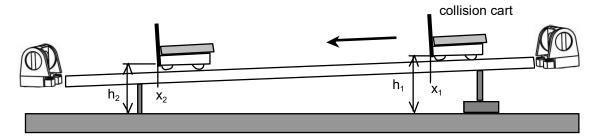
Figure 2. Illustration of position and height measurements on track. (the lower end of the track should be closer to the wall)
